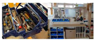
Before/after: Thanks to the reorganization, you no longer have to waste time searching for tools – everything is available directly! The workstations should be adapted ergonomically and individually for the activities performed. Methods such as kanban and the principle of easy accessibility help to achieve this goal.
